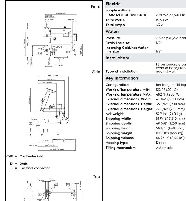
FS on concrete base;FS on feet;On base;Standing against wall Rectangular; Tilting 122 °F (50 °C) 482 °F (250 °C) 47 1/4" (1200 mm) 35 7/16" (900 mm) External dimensions, Height: 27 9/16" (700 mm) 529 lbs (240 kg) 51 9/16" (1310 mm) 49 5/8" (1260 mm) 58 1/4" (1480 mm) 1003 lbs (455 kg)
